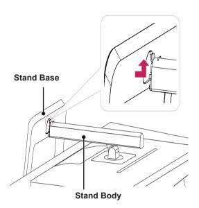
4 Fix by turning the screw to the right with a coin.
